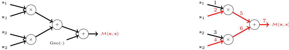
(a) Standard garbled circuit. The \epsilon -privacy budget is concentrated on mechanism output. (b) DP garbled circuit. The \epsilon -privacy budget is distributed across wires as well as mechanism output.
